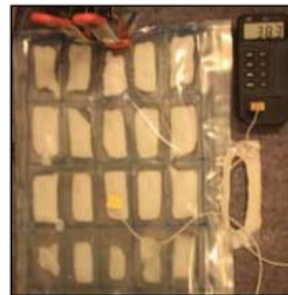
Fig 134: Checking pcm temperature
